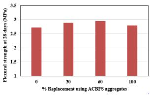
Fig. 5(b) –Flexural strength (28 days) of mixes with different Replacement Percentages of ACBFS aggregate
