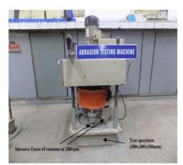
Fig. 9 - Revolving-disk abrasion test machine
