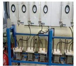
Fig. 8 - Test Setup for Water permeability test
