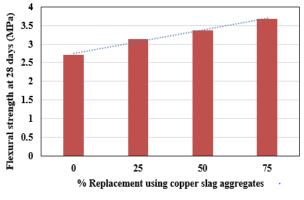
Fig. 3(b) –Flexural strength (28 days) of mixes with different Replacement Percentages of Copper Slag aggregate
