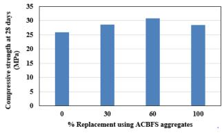
Fig. 5(a) –Compressive strength (28 days) of mixes with different replacement percentages of ACBFS aggregate
