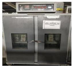
Fig. 7 – Carbonation Chamber for ACT
